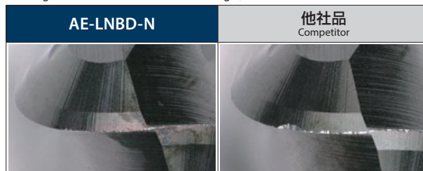
2,480m 加工後のボール部逃げ面摩耗状態 Wearing condition of ball flank after milling 2,480m
